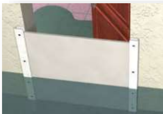
Figure 6: Installation de batardeaux
